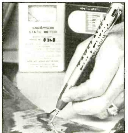
Be cautious with poly bags, which may have exposed carbon or metal on the surface—a shock or ESD hazard.
