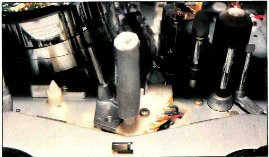
Figure 2. You can cover the tape sensor with a piece of cable jacket.
