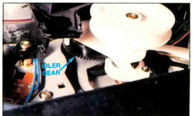
Figure 9. To move the gear into an area where it can clear the chassis, turn the idler gear assembly to the left.
