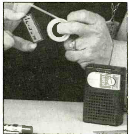
Even seemingly innocuous actions can develop a substantial static charge. Here, unrolling Scotch tape generates opposite charges on the roll and on the unrolled strip. Bringing the tape strip near an LED display causes a trickle of discharge through the LEDs, as shown by the lighting of some of the LED segments.
